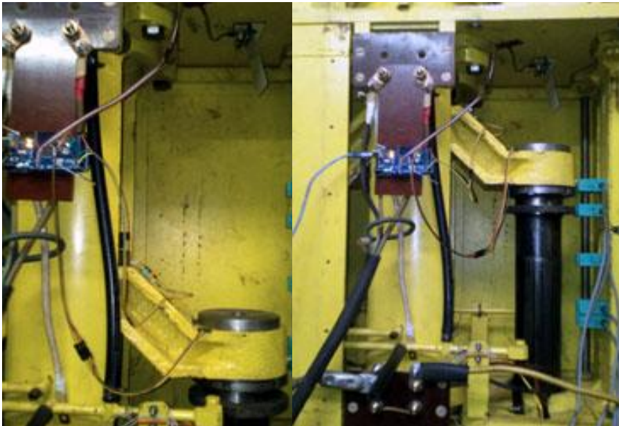
Fig. 4 - Photos of the installation of the Arduino Mega 2560 microprocessor controller and the HC-SR04 digital sensor on the prototype of the electromagnetic hammer.
