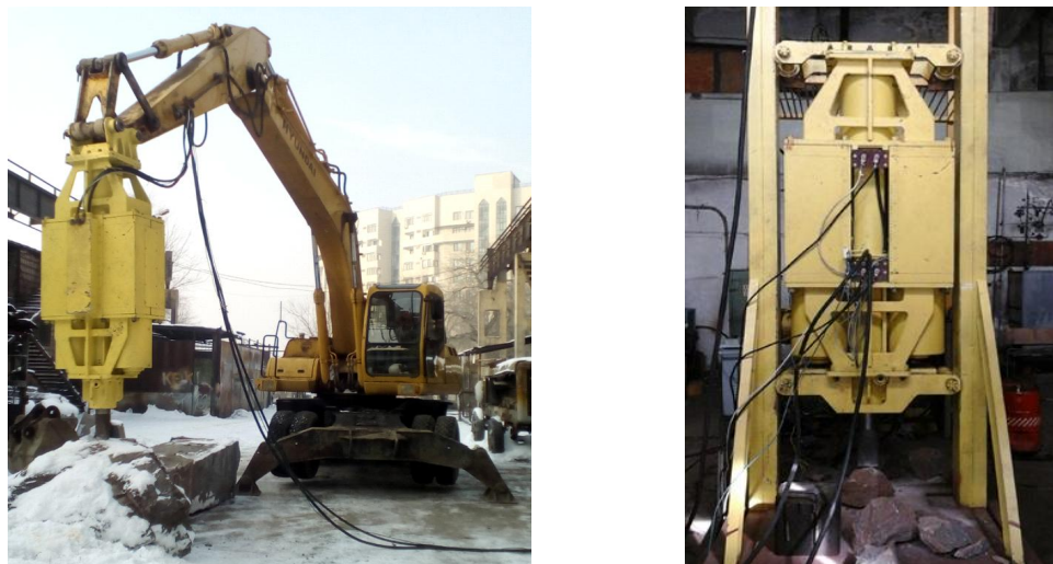
Fig. 1 - Photos of the EMH units as attachments on the HYUNDAI 210 wheel excavator and on a test bench equipped with a hydraulic lift
